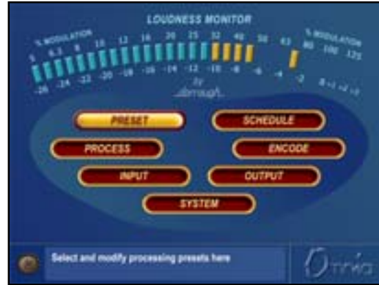
Main Menu display includes a Dorrough Loudness Meter for accurate peak-to-average measurements of final output.
